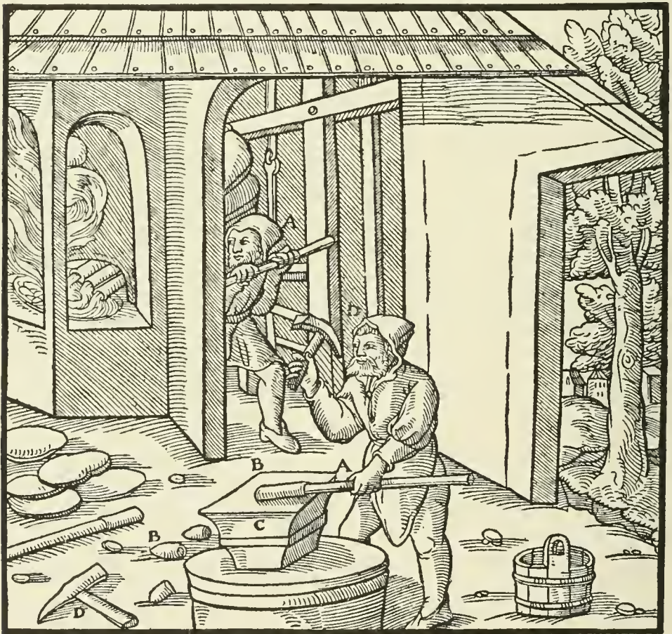
A—POINTED BAR. B—THIN COPPER LAYER. C—ANVIL. D—HAMMER.
